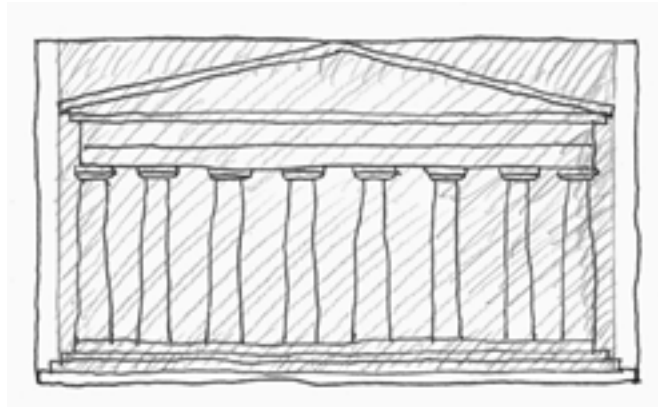
Figure 7. Some Golden Mean enthusiasts draw this shaded rectangle on the Parthenon's façade, using the bottom of the third step. Others only go to the bottom of the first step. Others still, use the bottom of the building's base (a thinner slab that is not a fourth step: there are only three marble steps) and width somewhere out in space.
